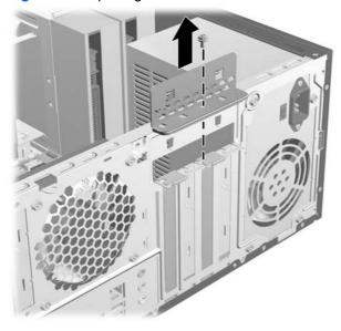
**8.** Before installing an expansion card, remove the expansion slot cover or the existing expansion card.
